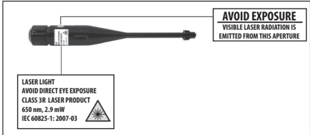
*Laser light is 650 nm, 2.9 mW, 0° beam divergence*
