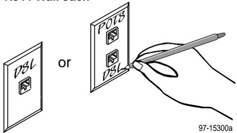
The RJ11 6-pin jack uses the center two pins. For pin assignments, refer to *Cables & Connectors* on page 14.
