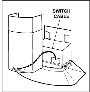
2. Slide the **lower decorative flue section** downward and into the **channels** on the hood.
