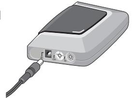
*Note* To avoid interference, the adapter cable should be kept away from the RF Extender as far as possible.
