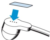
The more holes you seal with the sealing tape, the greater is the bass attenuation. This increases the speech intelligibility without increasing the volume – which is an advantage for people with a hearing impairment at high frequencies.
