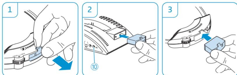
With a spare BA 151 rechargeable battery (to be ordered separately), you can use the A 200 for more than twice the time. You can charge the spare rechargeable battery while using the supplied one and replace one with the other when needed.
