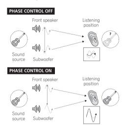
Phase Control technology provides coherent sound reproduction through the use of phase matching<sup>4</sup> for an optimal sound image at your listening position. The default setting is on and we recommend leaving Phase Control switched on for all sound sources.
