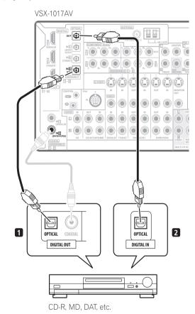
1 Connect an optical-type<sup>1</sup> digital audio output on your digital component to the DIGITAL 3 (CD) input. Use an optical cable for the connection.
