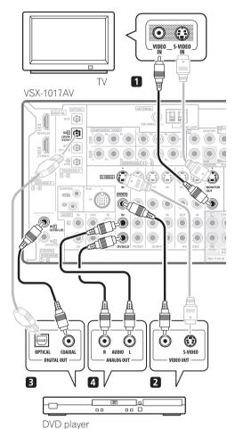
The diagram shows a basic setup of this receiver together with a TV and DVD player, with S-video or composite video connections. Different TVs and DVD players may offer alternative connections. See also *Using the component video jacks* on page 14 if your TV and/or DVD player has component video inputs/outputs. If your DVD player offers multichannel analog audio outputs, see *Connecting the multichannel analog inputs* on page 47.
