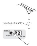
To improve AM reception, connect a 5 m to 6 m length of vinyl-coated wire to the **AM LOOP** terminals without disconnecting the supplied AM loop antenna.
