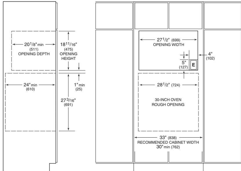
NOTE: At installation, wood cleats must be added to the opening for the microwave trim.
