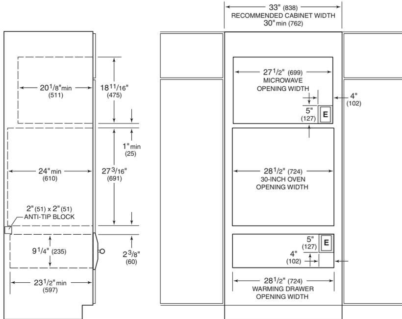
NOTE: Refer to the built-in 30" (762) single oven specifications for electrical location.
