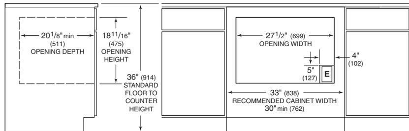
NOTE: At installation, wood cleats must be added to the opening for the microwave trim.
