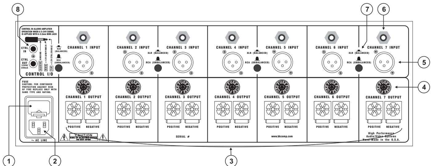
1. **AC Fuse Holder** - Holds the AC line fuse. This fuse is a 12 amp / 250 volt slow blow fuse. Replace only with the same type and value fuse.
