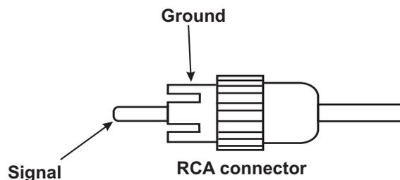
Use either RCA unbalanced or XLR balanced to connect the preamplifier to amplifier.
