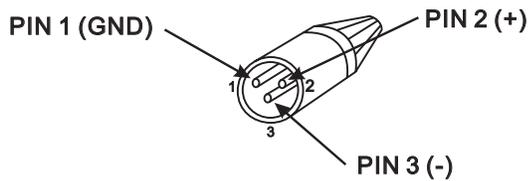
Amplifier Balanced Input Connector
