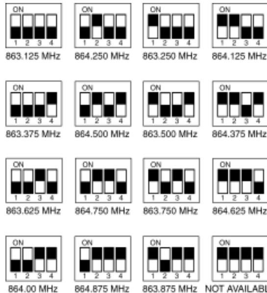
Set the dip switches on the receiver and the belt pack transmitter or hand held mic transmitter to matching frequencies. The dip switches for the receiver are located on the front panel. The dip switches for the belt pack transmitter are located on the side of the belt pack. The dip switches for the hand held mic can be accessed by opening the battery holder on the side of the mic.
