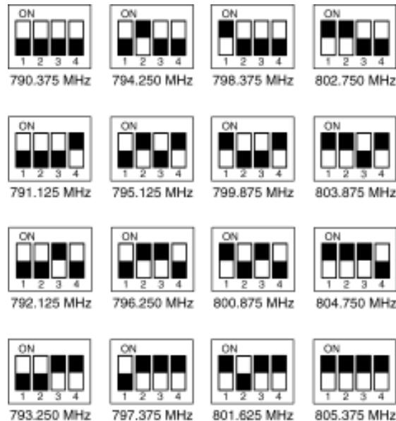
Set the dip switches on the receiver and the belt pack transmitter or hand held mic transmitter to matching frequencies. The dip switches for the receiver are located on the front panel. The dip switches for the belt pack transmitter are located on the side of the belt pack. The dip switches for the hand held mic can be accessed by opening the battery holder on the side of the mic.
