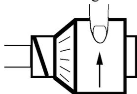
*Note: Failure to follow recommended stylus pressure could damage both the stylus and record. This can also seriously degrade performance.*
