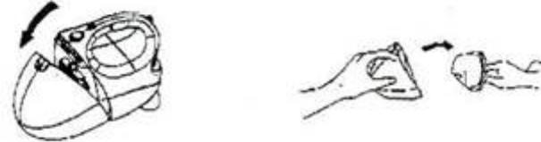
2. To use the Hand Vacuum with the shoulder strap (7), attach it to the unit as shown below.
