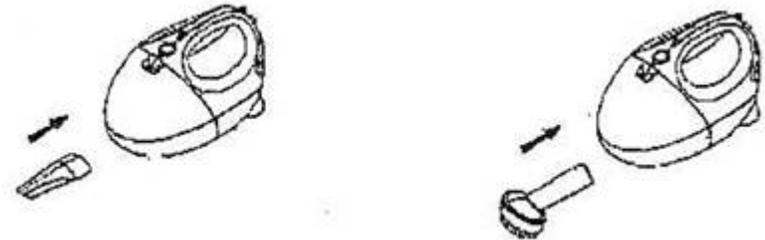
4. To use the flexible hose (11), push the end of the hose into the suction hole (3), then attach the desired brush (8 or 12) to the other end of the flexible hose (11), as shown below.
