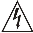
A triangle with a lightning symbol draws the user's attention to "dangerous voltage" without insulation in the cabinet which may be high enough to entail a risk of electric shock.
