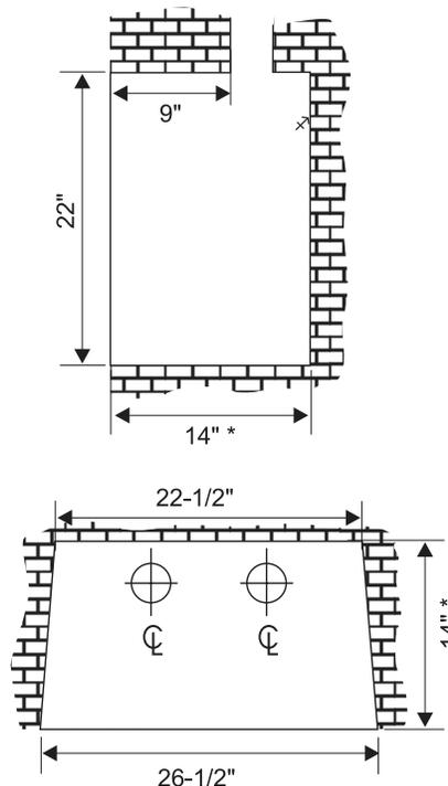
**\*Note: If you are installing the Molded Faceplate, the minimum fireplace dimensions are as follows:**
