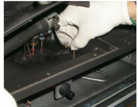
*Note: when installing the burner assembly be sure to slide the aeration adjustment wire through the hole in the base of the burner tray.*
