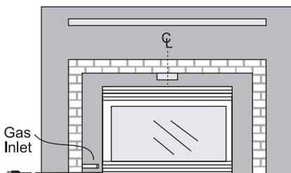
pass through the chimney above the appliance. Move the appliance into the exact location where it is to be installed. Ensure that the Insert is level.
