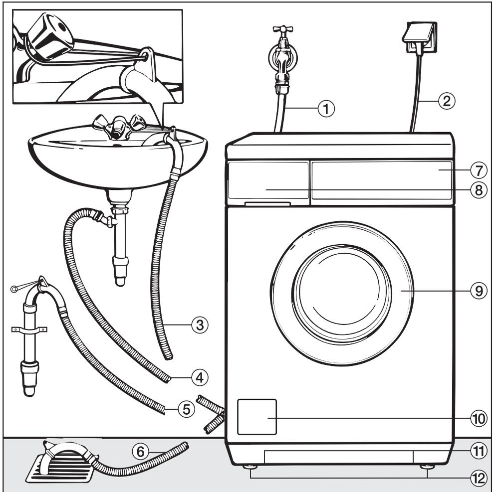
① Inlet hose (tested to withstand pressure of at least 7,000 kPa)
