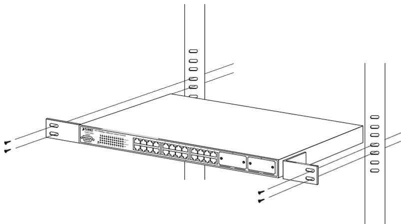
**Figure 2-6** Mounting the Switch in a Rack
