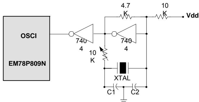
Fig. 33. Crystal/Resonator-Parallel Mode Circuit
