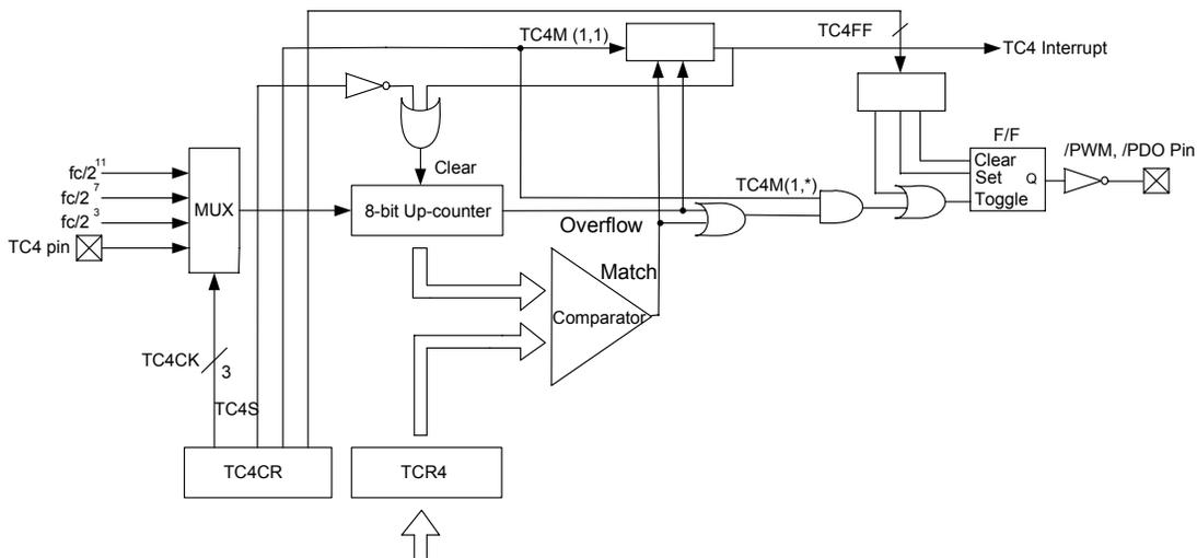
Fig. 25. Timer/Counter 4 Configuration
