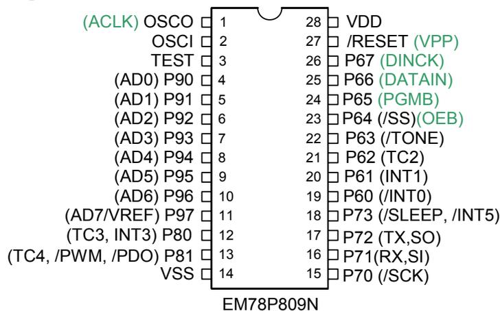
Fig. 1. Pin Assignment
