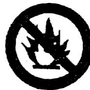
■ Always use extreme caution when working with **flammable** liquids. When refueling, **stop** the engine and allow it to cool. **DO NOT** smoke around or near the machine. Fire or explosion could result from fuel vapors, or if fuel is spilled on a hot engine.
