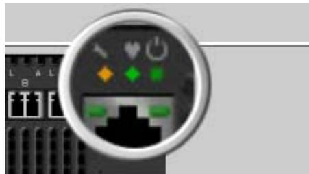
**Figure 4-14. Hardware Status LEDs**
