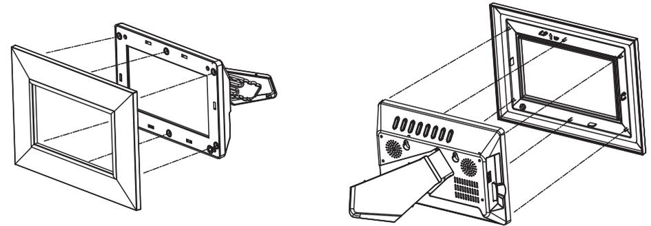
Please note that removal and installation of the faceplate is easy. Please refer to the above illustration for removing and installing the faceplate.
