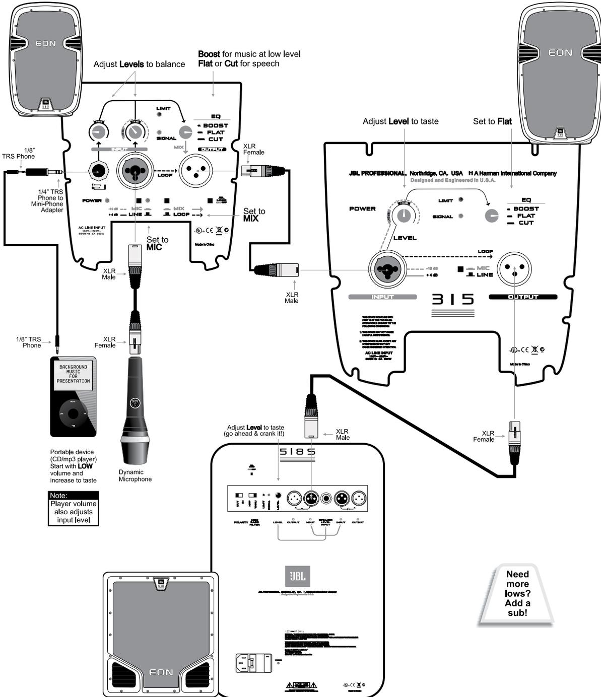
PA Using Powered Mixer And Powered Subwoofers
