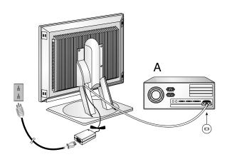
The AC adapter and signal cable are connected to your monitor. If you wish to change these or to fit a different stand, see Further Help on page 22.
