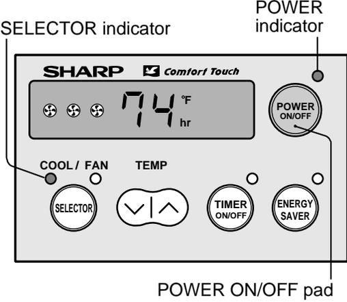
The diagram shows the control panel with the following components labeled: SELECTOR indicator, POWER indicator, SHARP Comfort Touch logo, a digital display showing 74°F and hr, COOL / FAN indicator, TEMP indicator, SELECTOR pad, POWER ON/OFF pad, TIMER ON/OFF pad, and ENERGY SAVER pad.
