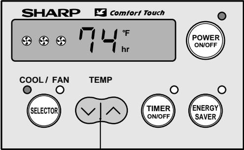
The diagram shows the control panel with the following components labeled: SHARP Comfort Touch logo, a digital display showing 74°F and hr, COOL / FAN indicator, TEMP indicator, SELECTOR pad, POWER ON/OFF pad, TIMER ON/OFF pad, ENERGY SAVER pad, and the TEMPERATURE setting pad (with up and down arrows).
