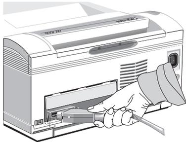
2. Plug the power cord into the printer, then into a grounded outlet.
