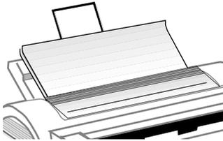
Pull out the rear exit extender until it locks into place. Lift out the metal support bar.
