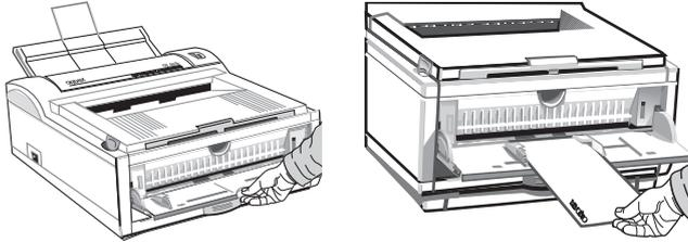
1. Pull out the rear exit extender until it locks and lift out the support bar. Pull down the manual feed tray and adjust the paper guides.
