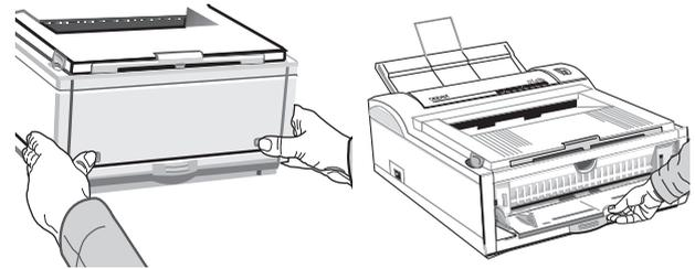
2. Adjust the guides. Insert a sheet of paper until the printer grips it. When using letterhead paper, insert letterhead in first, face up.
