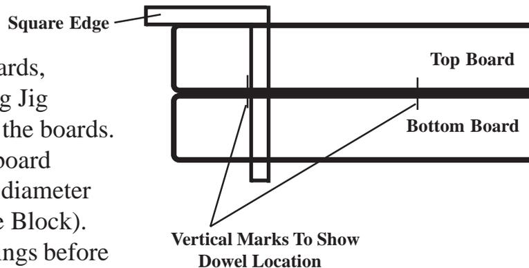
3. With the dowel holes precisely drilled, it is easy to assemble the two boards together. Put glue in the holes and on the dowels. Insert the dowels into the holes and tightly clamp the boards until glue has dried.
