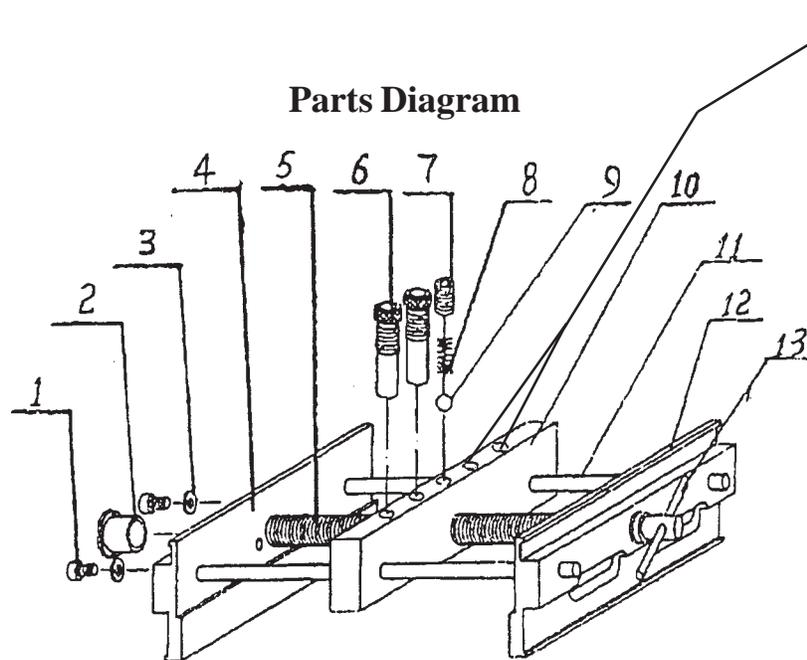
**Note:** There are 4 holes along the top of the Jig. Only 2 of the holes accept threaded bushings. The other 2 holes accept 7/16" and 1/2" drill bits.
