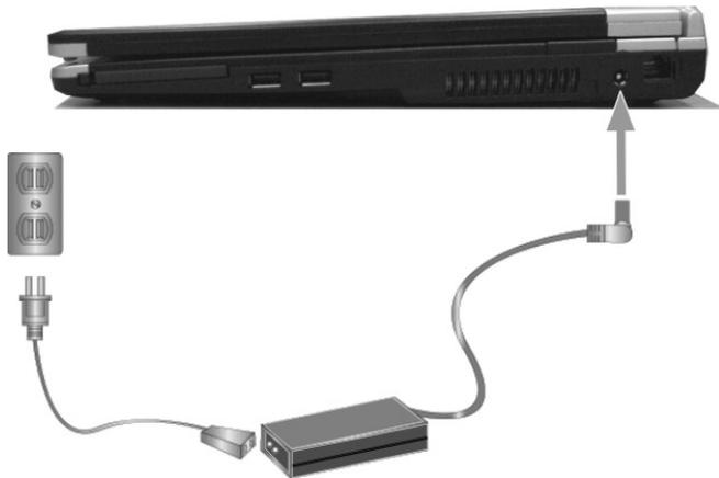
3. Plug the connector of the AC adapter to the DC-IN port found at the Right side of the computer.
