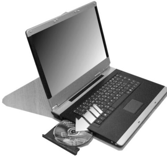
3. To remove the disc, press on the center spindle and pull up the disc from the side until the disc snaps out of the spindle lock.
