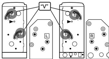
Set "V" for all the four angle adjustment parts on both sides.
