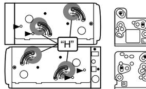
Set "H" for all the four angle adjustment parts on both sides. Cover the holes indicated by "▶"/"○" with the dustproof seals ⑪, ⑫. Use the holes marked "●" to install the unit.
