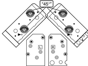
Set "45°" for all the four angle adjustment parts on both sides.
