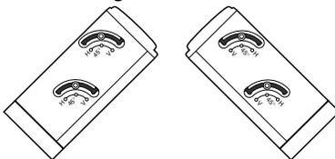
The angle adjustment switches on the both side of the unit are to be set according to the angle of installation of the DVD/CD auto changer. Set both of the 4 switches to the same position. If the switches are not set properly, sound skip or other malfunction may occur.
