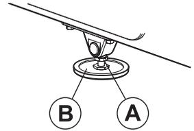
After placing the unit where it will be used, check its stability. If there is even a slight rocking motion or the unit is not stable, determine which stabilizing leg is not resting on the floor. To adjust, loosen the JAM NUT (A), and turn the STABILIZING LEG (B) until the rocking motion ceases, and both stabilizing legs rest firmly on the floor. Retighten the JAM NUT.
