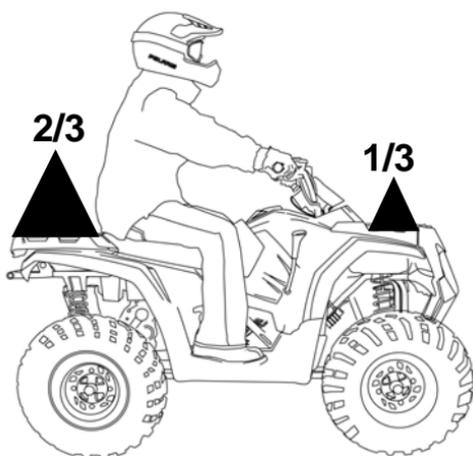
Your ATV has been designed to carry or tow a certain amount of load. Always read and understand the load distribution warning labels on the vehicle, and never exceed the weight capacities outlined in the specifications section of the owner's manual and on the safety decals.
