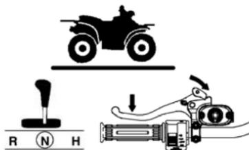
4. Start the engine. Allow it to idle for two to three minutes. Stop the engine.
