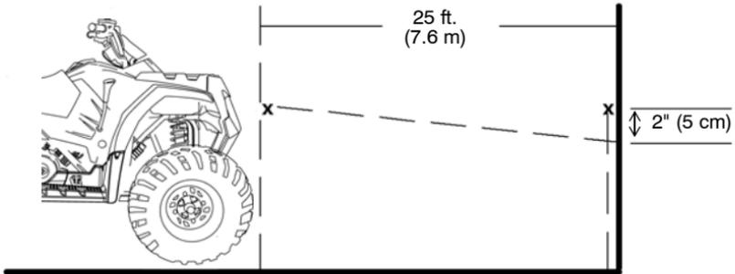
1. Position the vehicle on a level surface with the headlight approximately 25 ft. (7.6 m) from a wall.
