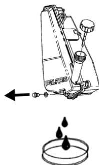
9. Reinstall the oil tank drain plug.
