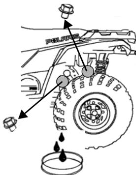
8. Clean and reinstall the drain plug. Torque to specification. See page 78 for recommendations.
