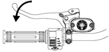
Always test brake lever travel and master cylinder fluid level before riding. When squeezed, the lever should feel firm. Any sponginess would indicate a possible fluid leak or low master cylinder fluid level, which must be corrected before riding. Contact your dealer for proper diagnosis and repairs.
