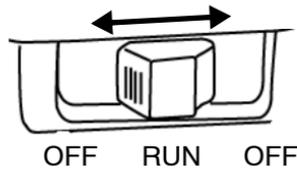
**NOTE:** Both the main switch and the engine stop switch will shut off all electrical power to the vehicle, including lights.
