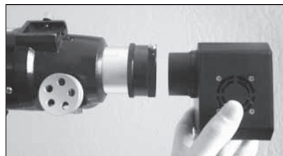
Figure 5.1. The Parsec fits into a 2" focuser, just like a standard 2" eyepiece. Firmly tighten the thumbscrew that secures the Parsec in the focuser.
