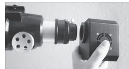
Figure 5.2. If your telescope has T-threads, remove the nosepiece from the Parsec and thread the camera directly onto the telescope. This provides the most secure connection.
