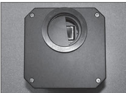
Figure 3.1. The shutter is free to move when the Parsec is off.
