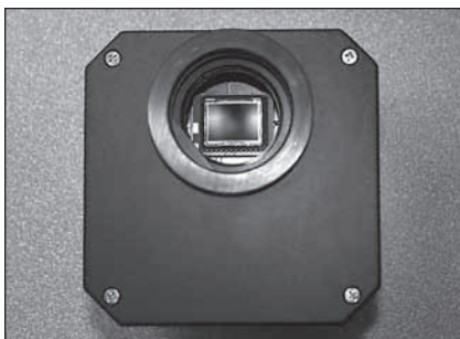
Figure 3.2. The shutter resets its position and holds firmly in place when the Parsec is powered on.
