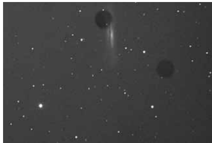
Figure 21.2. Dust or other particles on the camera's optical window can show up as distracting dark shapes in your images.
