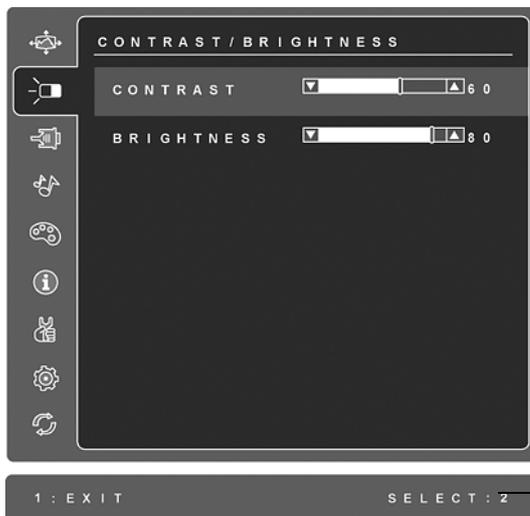
The line at the bottom of the screen shows the current functions of buttons 1 and 2: Exit or select the control.
