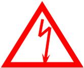
The lightning flash with arrowhead symbol, within an equilateral triangle, is intended to alert the user to the presence of uninsulated "dangerous voltage" within the product's enclosure may be of sufficient magnitude to constitute a risk of electric shock to persons.
