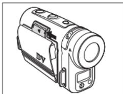
Your DV camera can also use alkaline batteries instead of a single rechargeable Lithium ion battery. Four AAA-sized alkaline batteries should be used in place of the supplied rechargeable Lithium ion battery and should be inserted as shown.
