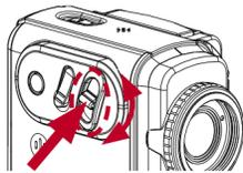
3. Press **Shutter** halfway to focus picture and completely down to take a picture.
