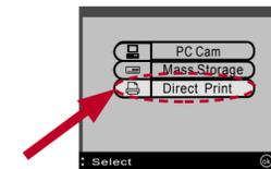
4. Press **OK** on the **Direction Control** to confirm the device is connected to a printer.
