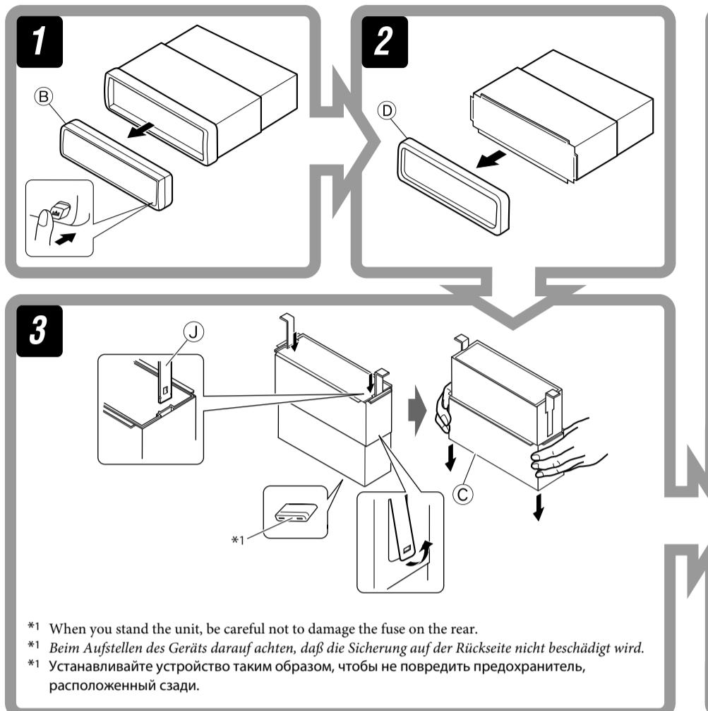
\*1 When you stand the unit, be careful not to damage the fuse on the rear.
