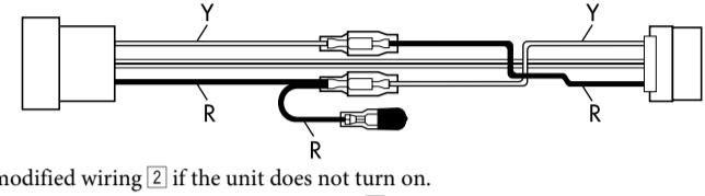
Use modified wiring 2 if the unit does not turn on.
