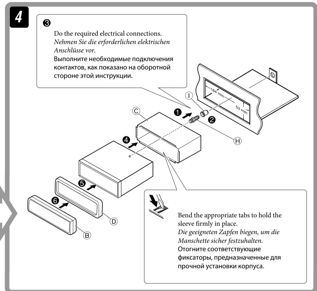
Bend the appropriate tabs to hold the sleeve firmly in place.
