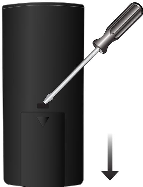
Insert a flat-head screwdriver into the slot as shown. Gently push down on the tab, then press and pull downward on the battery cover to open.
