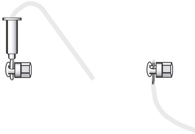
● Contacts for the INPUT connectors are wired in parallel. This makes it convenient when a parallel connection is desired. (Parallel Connection → p. 9)
