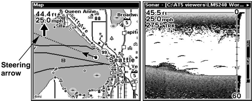
At left, Map Page showing boat cruising Puget Sound, Washington, with Overlay Data turned on. This example shows Depth, Ground Speed and the Steering Arrow. Note that the Steering Arrow always points directly to the destination you are navigating toward. In this case, the boater is headed on a northwesterly course of 275°. Since the helmsman is on course, the Steering Arrow is pointing straight ahead.
