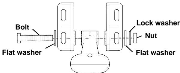
Assemble transducer and bracket.
