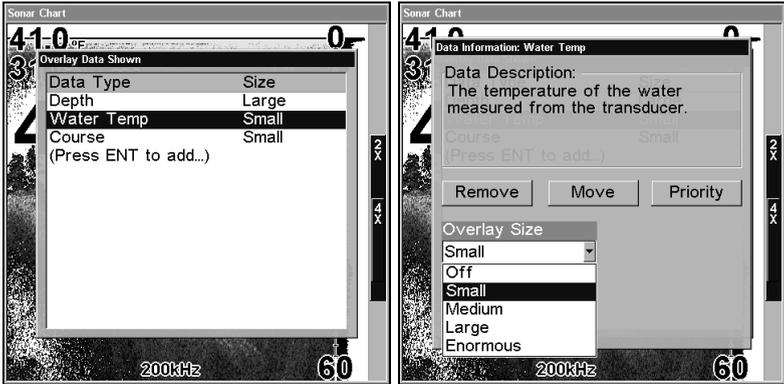
Left, Water temp in the overlay data shown menu. Right, the overlay data size window. Notice the water speed data description at the top of the data information window.
