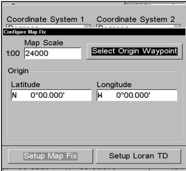
**Configure a map fix so the unit can find your position on a printed chart or topographical map.**
