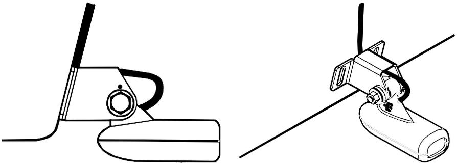
For single-frequency Skimmer, route cable over bolt and through bracket. Side view shown, left, and seen from above at right.
