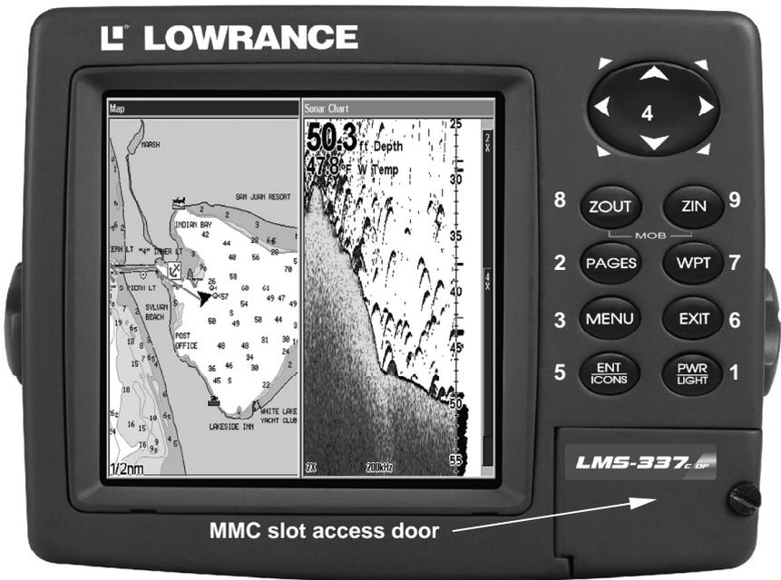
LMS-337CDF sonar/GPS unit, front view, showing map with sonar split screen, keyboard and access door for the MMC slot.
