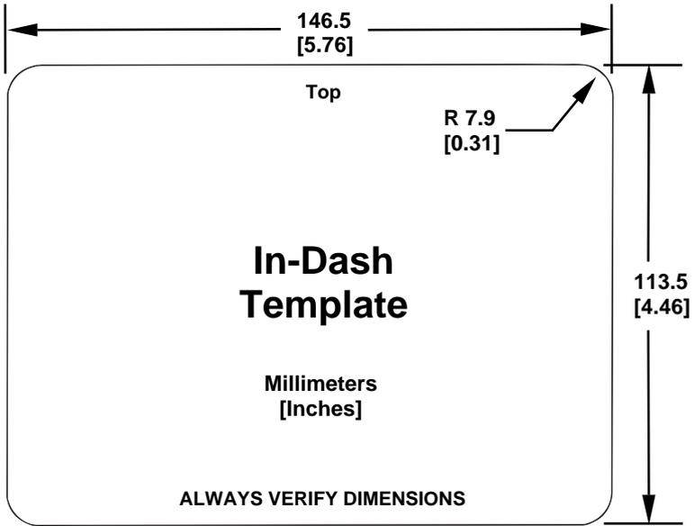
**In-dash mounting template for LMS-332 and LMS-337CDF sonar/GPS units, showing dimensions.**
