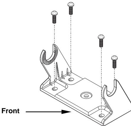
**Install the gimbal bracket. Orient the bracket so the arms slope toward the front of your unit.**
