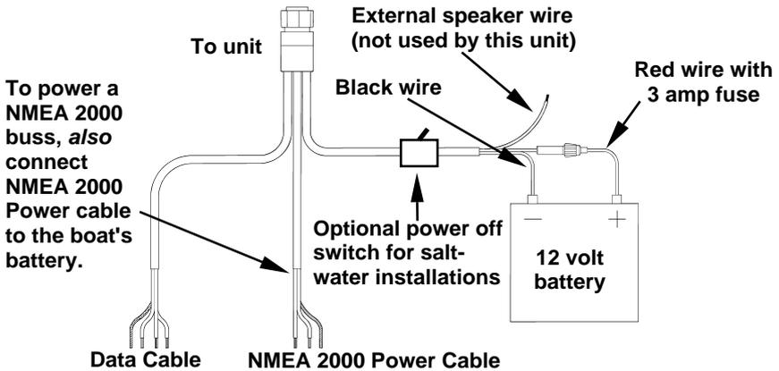
Power connections for LMS-332 and LMS-337CDF sonar/GPS units.
