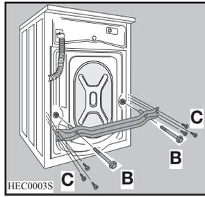
5. Remove the bracket **D** and tighten up the six smaller bolts **C**.
