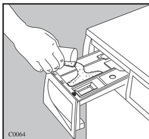
If required, pour fabric softener into the compartment marked
