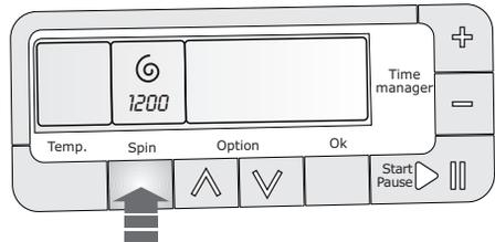
Press the Spin button repeatedly to change the spin speed, if you want your laundry to be spun at a speed different from the one proposed by the washing machine.
