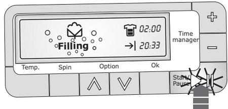
To start the selected programme, press the “Start/Pause” button; the green pilot light stops flashing. On the display will appear the icon, and alternatively the name and the running phase of the selected programme to indicate that the appliance starts
