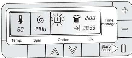
**Prewash:** select this option if you wish your laundry to be prewashed before the main wash (not available for wool, handwash, silk, blanket and 14 min programmes). The Prewash ends with a short spin at 650 rpm in programmes for cotton and synthetic fabrics, whereas in the program for delicate fabrics the water is only drained.
