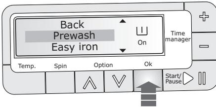
Once you have completed the selection of the options, press «Temp» or «Spin» buttons or simply wait 10 seconds to return the display in the default status. The selected icons will be shown on the display.
