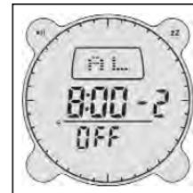
The alarm can also be turned on or off by going to the relevant alarm and pressing the **COMP** button to activate alarm function, press again to activate Snooze function, and press again to de-activate alarm.
