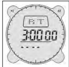
Press any button when alarm sounds to stop the Countdown Timer. If nothing is pressed the Countdown Timer will stop beeping after 10 seconds, but it will continue if the 'AUTO' function is set on. To stop the Countdown Timer if the 'Auto' function is on, you must go to the Countdown Timer Mode and press **COMP** to turn off the 'Auto' function and then press **UP** button to stop it.
