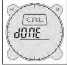
will then go automatically into Declination Setting Mode. If Calibration is unsuccessful, the Cardinal Points will blink and you will have to repeat the previous 4 steps again. To skip setting the declination, press the **ADJ** button to return to the Compass Mode.
