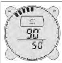
To operate the compass in Homing Mode go into the Compass Mode first, then press **MODE** button to get into Homing Mode.
