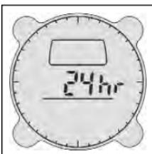
For 24/12 hour setting press **MODE** button until Time Mode is displayed. Press and hold down **ADJ** for 3 seconds. Press **MODE** button and scroll through settings until 24/12 hour setting appears, then press **UP** or **DOWN** button to enter desired setting. Press **ADJ** button at any time to save changes and exit.
