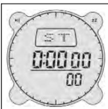
For split timing function, press the **DOWN** button while the Stop Watch is operating in order to stop the display and press again to continue. You can also press the **DOWN** button while the Stop Watch is operating to stop the display and then press the **UP** button to stop the Stop Watch and display the final reading. Press the **DOWN** button again to reset the Stop Watch.
