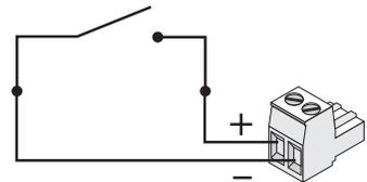
**Logic Out connections. Negative (-) terminal is at chassis potential. Positive (+) terminal logic level is switched using software.**
