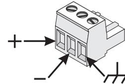
**Analog audio input- unbalanced connection. Note jumper wire between - and ground.**
