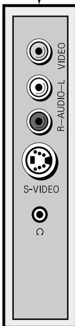
On the right side panel of the HDTV Monitor, you will find the Video 3 inputs and Headphone jack. These are provided to connect a camcorder or other video equipment without reaching around to the rear panel.
