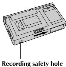
Recording safety hole
