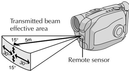
When using the remote control, be sure to point it at the remote sensor. The above illustration shows the approximate transmitted beam effective area for indoor use. The transmitted beam may not be effective or may cause incorrect operation outdoors or when the remote sensor is directly exposed to sunlight or powerful lighting.
