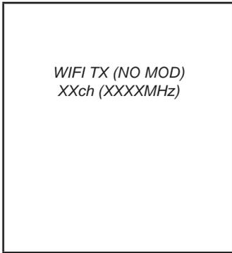
5. In this state, each time the [VOL +]/[VOL -] keys are pressed, the transmission channel is changed.
