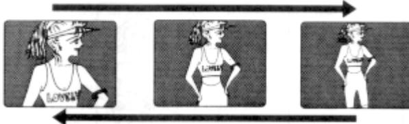
When the power zoom switch is operated, the zoom position is displayed in the viewfinder for about 5 seconds and then disappears. The zoom position is displayed in 10 steps.
