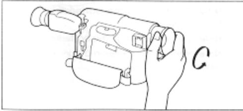
2. Remove both caps of the converter lens.
