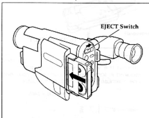
3. Push the cassette holder, which is embossed PUSH LOCK on the left hand side, until it "clicks" into place. The camcorder automatically closes.
