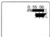
This flashing symbol indicates a battery nearly out of power. Use an alternate power source or charge the battery before continuing to use the camcorder.
