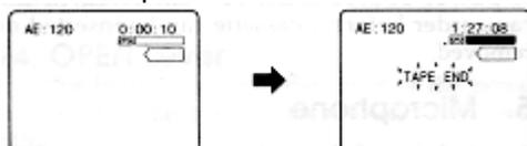
**Note:** The tape remaining display appears 10 seconds after the tape starts to run.
