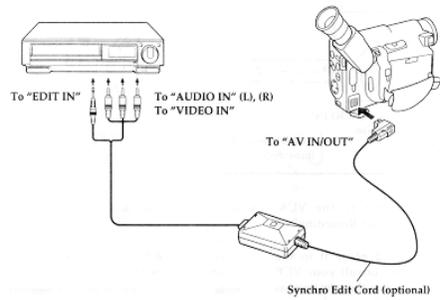
1. Connect the provided AV stereo output cable to the AUDIO IN and VIDEO IN jacks of your VCR. Connect either the right or left audio plug into your VCR if it has only one AUDIO IN jack.
