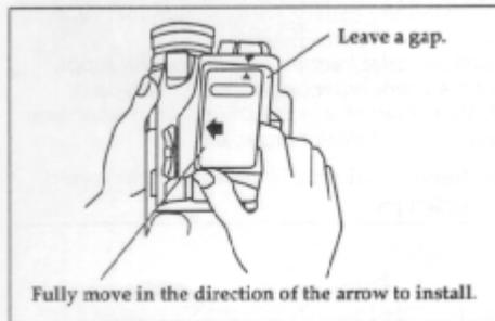
3. Once the arrows are aligned, push down on the battery.
