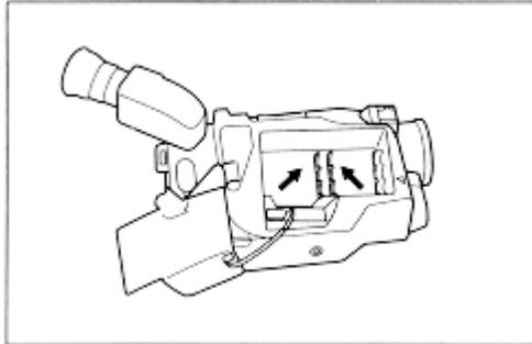
3. Insert six alkaline batteries with the correct polarities.
