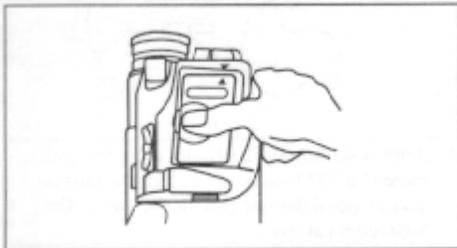
4. While pushing down the battery, slide it to the right until it "clicks" into place.
