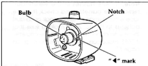
3. Install the new bulb by aligning the notch in the rim of the bulb's base with the "◀" mark outside the socket. Avoid touching the bulb directly with your fingers. It may shorten the life of the bulb.
