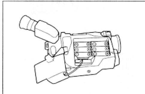
4. After installing the batteries, close the cover. Hold the OPEN lever and align the tabs on both sides of the cover with the end of the attachment section.
