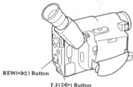
**Note:** When you engage F.F button or REW button the picture will have some interference or noise. This is normal during search mode.
