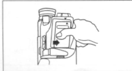
5. After installing the battery, close the cover. Hold the OPEN lever and align the tabs on both sides of the cover with the end of the attachment section.
