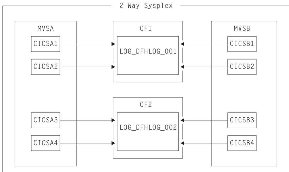
Figure 8. Sharing system logger structures between 2 MVS images
