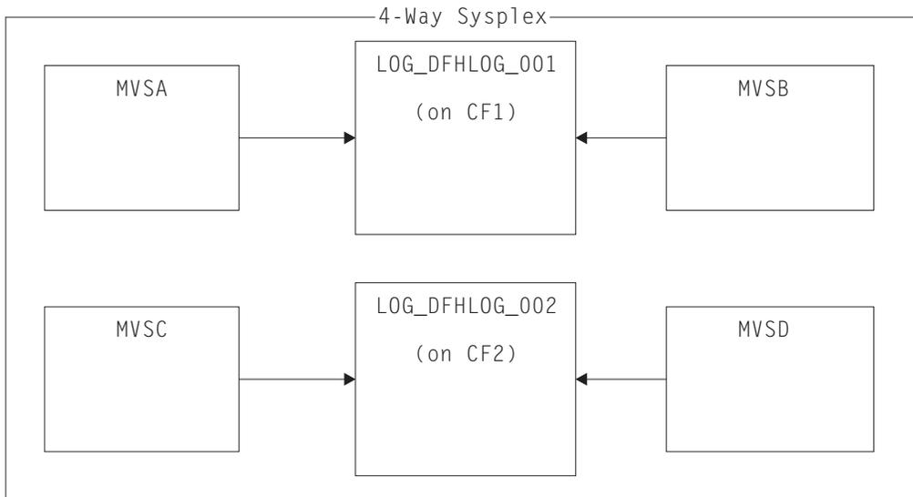
Figure 9. Sharing system logger structures between 4 MVS images
