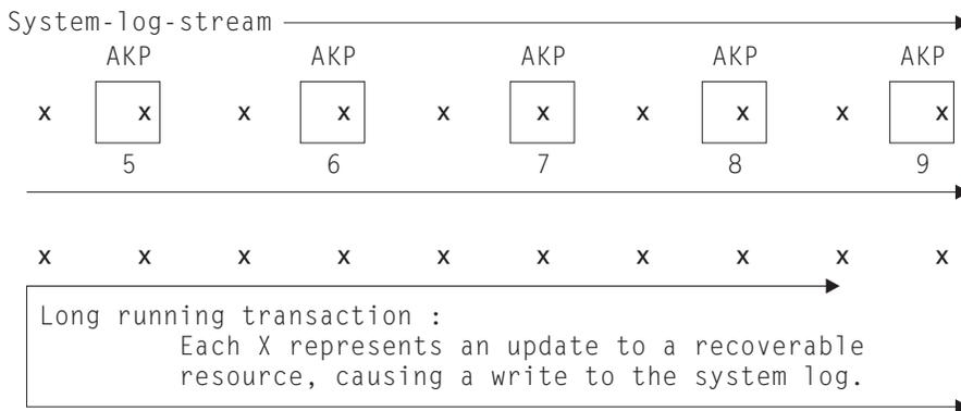
Figure 11. The effect of a 'bad' long-running transaction
