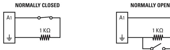
**Figure 11.** Supervised Alarm Input Wiring
