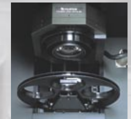
FUJINON lens VRF43LMD and five-position filter turret
