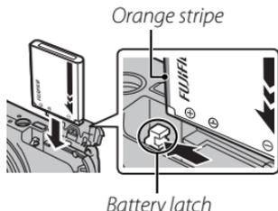
① Insert the battery in the correct orientation. **Do not use force or attempt to insert the battery upside down or backwards.** The battery will slide in easily in the correct orientation.
