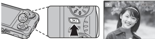
Press the selector right to view pictures in the order recorded, left to view pictures in reverse order. Keep the selector pressed to scroll rapidly to the desired frame.
