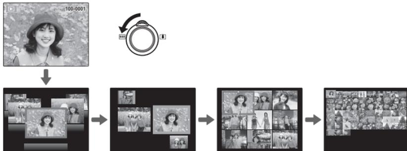
When two or more images are displayed, use the selector to highlight images and press **MENU/OK** to view the highlighted image full frame. In the nine- and hundred-frame displays, use the selector to view more pictures.
