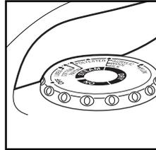
4. To turn iron Off, turn Temperature Control Dial to Off and unplug iron.
