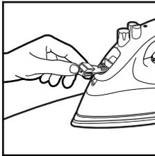
2. Using a cup, slowly pour 6 ounces of tap water into water tank opening. Do not fill iron directly from the faucet.
