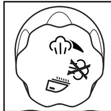
7. To turn iron off, set Adjustable Steam Knob to ☒ (Dry Iron). Turn the Temperature Control Dial to Off. Unplug iron.
